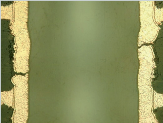
PTH barrel crack
