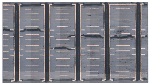
cross section of coupon showing delamination
