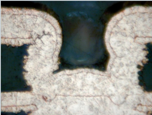
Microvia corner crack
